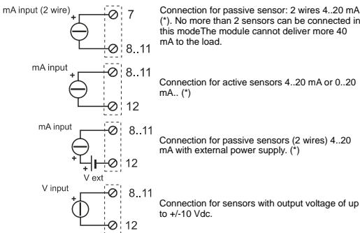
Connection for passive sensor: 2 wires 4...20 mA (\*). No more than 2 sensors can be connected in this mode! The module cannot deliver more 40 mA to the load.
