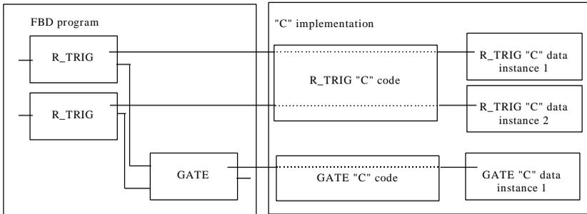
The memory needed for data structure of each instance is allocated by the ISaGRAF system, when the application starts. A pointer to the associated instance data structure is passed to the "activate" and "read" services.
