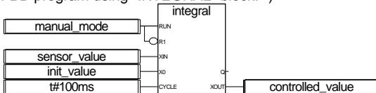
(\* ST Equivalence: INTEGRAL1 instance of INTEGRAL block \*)
