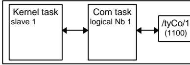
The most basic configuration consists in a kernel task associated to a communication task on a serial (Ethernet) link.
