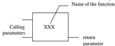
A "C" function can be called from any **SFC** action block, or in any boolean condition attached to a transition.
