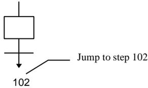
A jump symbol cannot be used to represent a link from a step to a transition. Example of jumps - the following charts are equivalent:
