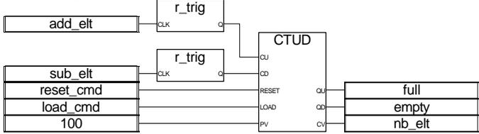
(\* ST Equivalence: We suppose R\_TRIG1 and R\_TRIG2 are two instances of R\_TRIG block and CTUD1 is an instance of CTUD block\*)
