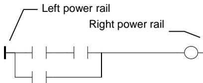
LD diagram graphic symbols are connected to power rails or to other symbols by **connection lines**. Connection lines are horizontal or vertical.
