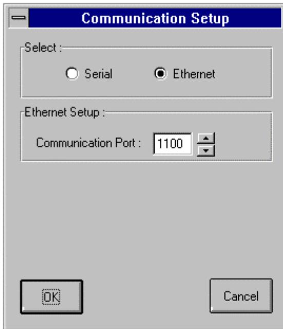
It is possible to choose the serial communication or the Ethernet communication. The Ethernet communication gives the possibility to modify the port number. This port number should be the same as in the workbench PC-PLC Link specification.
