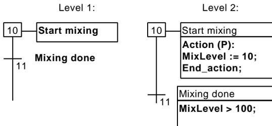
The level 2 programming of a step is entered in a text editor. It can include action blocks programmed in ST or IL. The level 2 programming of a transition can be entered either in IL or ST text languages, or with Quick LD editor.
