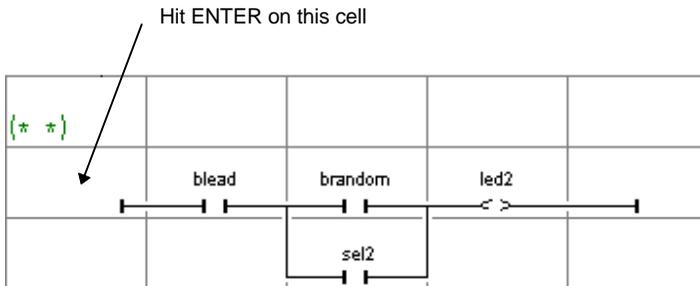
The ISaGRAF Quick LD editor keeps the memory of the rung labels you already entered, whether it has been specified for a rung name or a jump operation. The "Jump/Label" dialog box gives you the possibility either to enter a new label, or to select an existing one.
