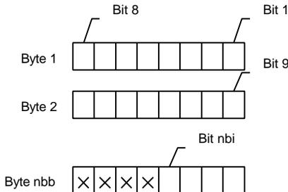
Bit 1 correspond to the value of the variable at addH/addL network address.
