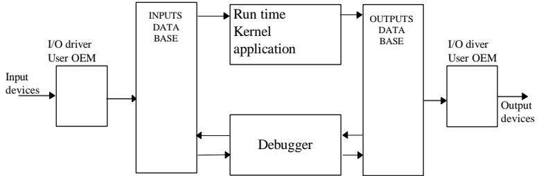
When an input variable is locked, the various accesses to the database are not changed, but the input device is disconnected. Input values can be set with the debugger and processed by the ISaGRAF kernel:
