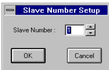
Using the mouse or the arrows (Up and Down) it is possible to change the value of this option. In order to use it, the ISaGRAF NT target should be restarted.
