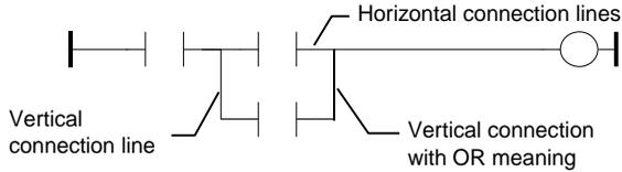
Each line segment has a boolean state **FALSE** or **TRUE**. The boolean state is the same for all the segments directly linked together. Any horizontal line connected to the left **vertical power rail** has the **TRUE** state.
