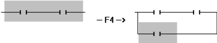
To insert symbols in the diagram, you can also use the commands of the "Insert" menu. With the mouse, you can click on the LD toolbar, on the type of symbol you want to insert:
