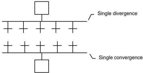
**Warning:** The conditions attached to the different transitions at the beginning of a single divergence are **not implicitly exclusive**. The exclusivity has to be explicitly detailed in the conditions of the transitions to ensure that only one token progresses in one branch of the divergence at run time. Below is an example of single divergence and convergence:
