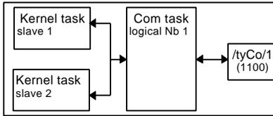
Another configuration consists in 2 kernel associated to a communication task on a serial (Ethernet) link. In this case, SlavesLink = 0x01020000.
