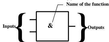
Input variables of an FBD program must be connected to input connection points of function blocks. The type of each variable must be the same as the type expected for the associated input. An input for FBD diagram can be a **constant** expression, any **internal** or **input** variable, or an **output** variable.
