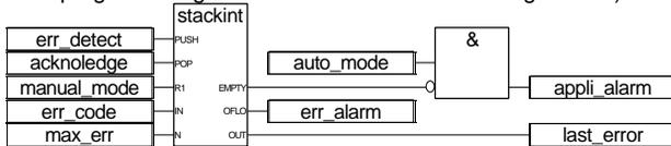
(\* ST Equivalence: We suppose STACKINT1 is an instance of STACKINT block \*)
