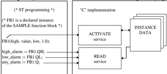
Because the "read" service can be called more than once in the same cycle, for the same return parameter or the same function block instance, no special calculation has to be performed in such a service. It only operates transfer between hidden data and the ISaGRAF application. Below is the standard frame of the read service:
