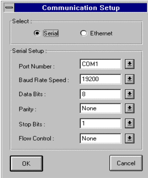
By choosing the serial communication, the configuration will appear. This configuration should be the same as in the workbench PC-PLC Link specification.
