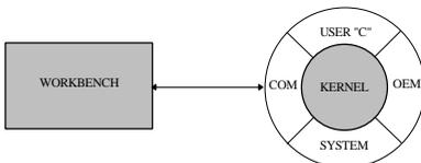
The inner part of ISaGRAF software is independent of the hardware. It executes the IEC languages and has its own variable data base.
